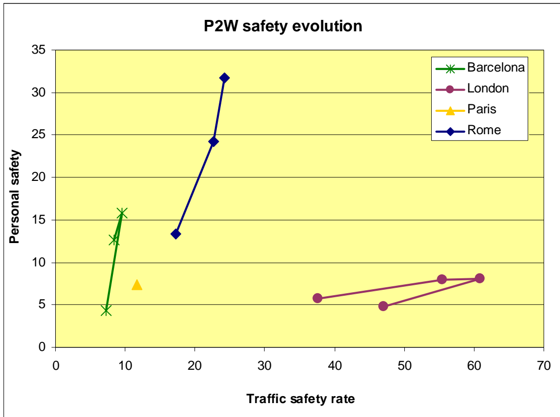
Figure 5.9 PTW safety evolution as personal safety (PTW fatalities per million inhabitants) versus traffic safety rate (PTW fatalities per 100,000 vehicles)
